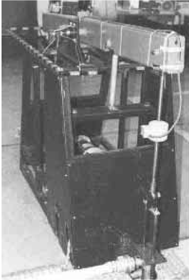
Figure 31: Piston pump with d.c. drive motor
