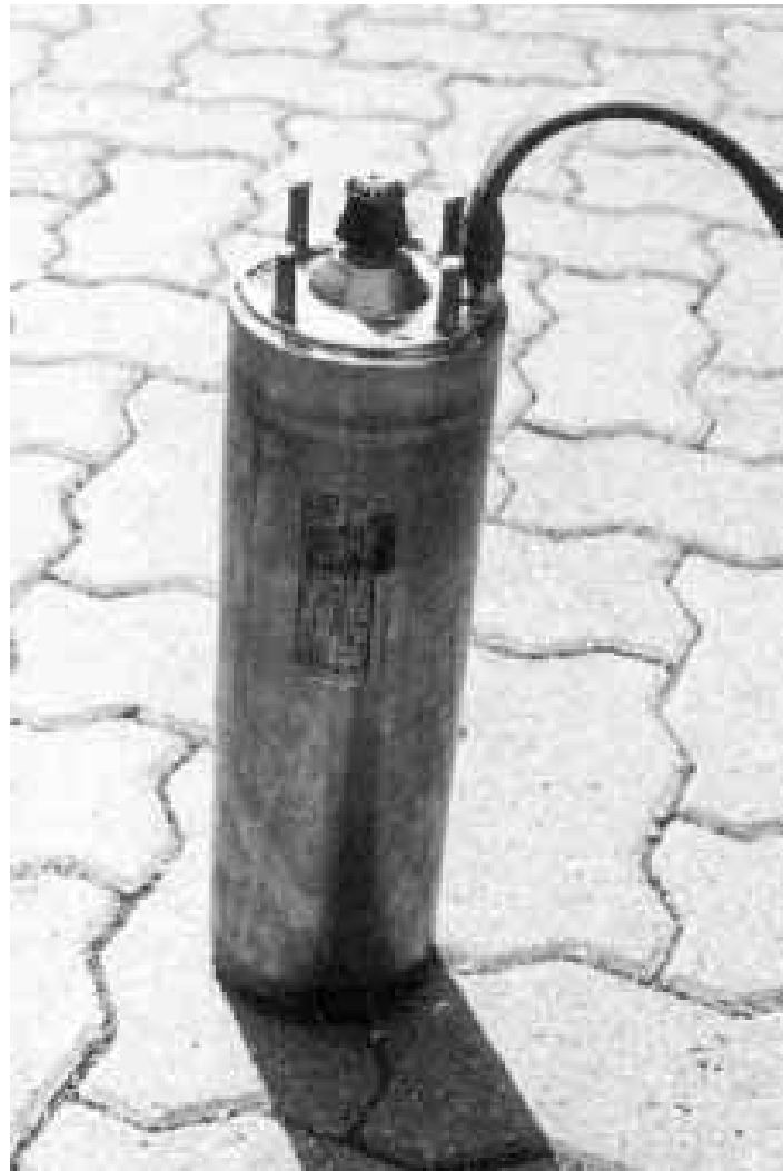
Figure 24: Standard asynchronous motor for borehole pumps
