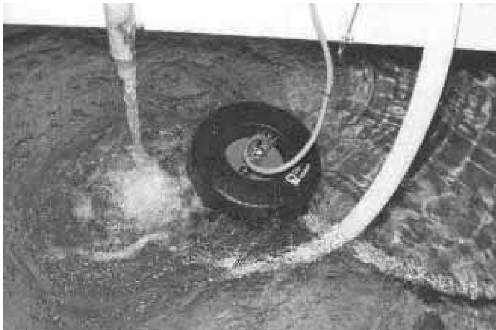
Figure 23: Floating pump with brushless d.c. motor
